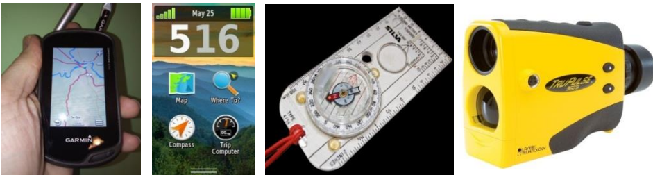
Fig. 3. User interface for GPS device GARMIN, hand-held bushing SILVA and TruPulse handheld laser rangefinder
