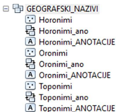
Fig. 1. Organization of object classes in the dataset GEOGRAFSKI_NAZIVI (screenshot captured in ESRI ArcMap 10.3.1) (MGI, 2024)
