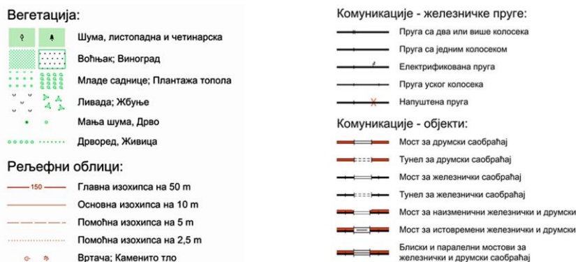
Fig. 9. An example for Topographical Key from 2015, Sheet Žagubica TK 25, 4 th edition, 2015
