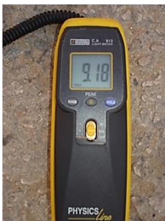
Fig. 5. The measuring instrument used a C.A 813 luxmeter (Source: Author)
