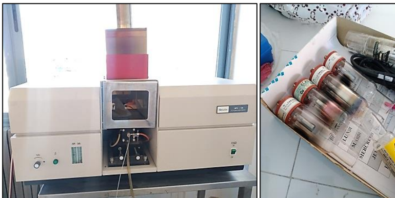
Fig. 5. Atomic Absorption Spectrophotometer (AAS) and its corresponding hollow cathode lamps used for trace metal analysis 6
